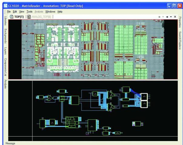
Fig.9 Illustration the ability of cross reference between layout and schematics
