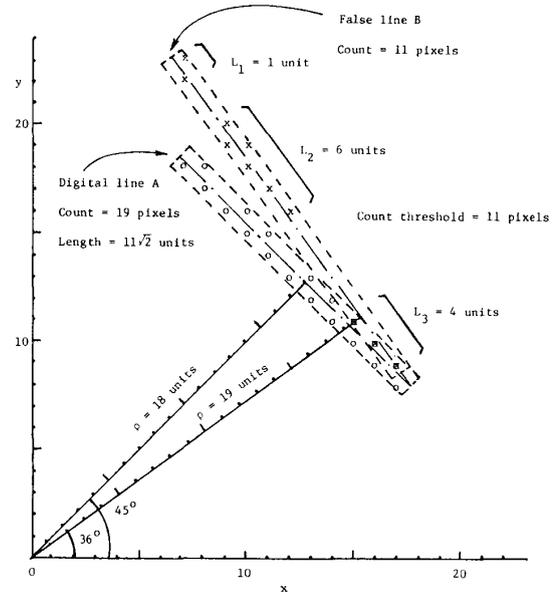
Fig. 2. Illustration of detection of digital line segments by the conventional Hough transform procedure.
