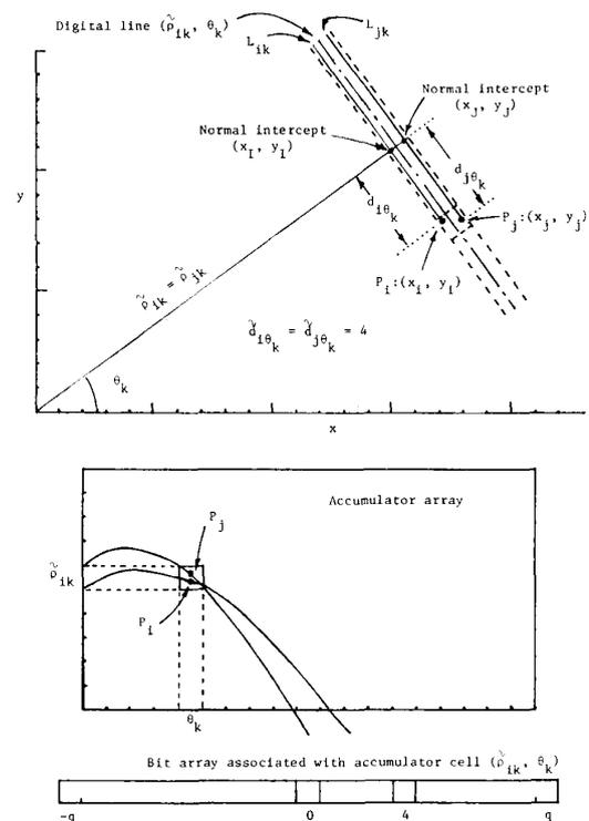
Fig. 3. Use of a bit array for controlling the count of accumulator cell to reflect the length of a digital line segment.
